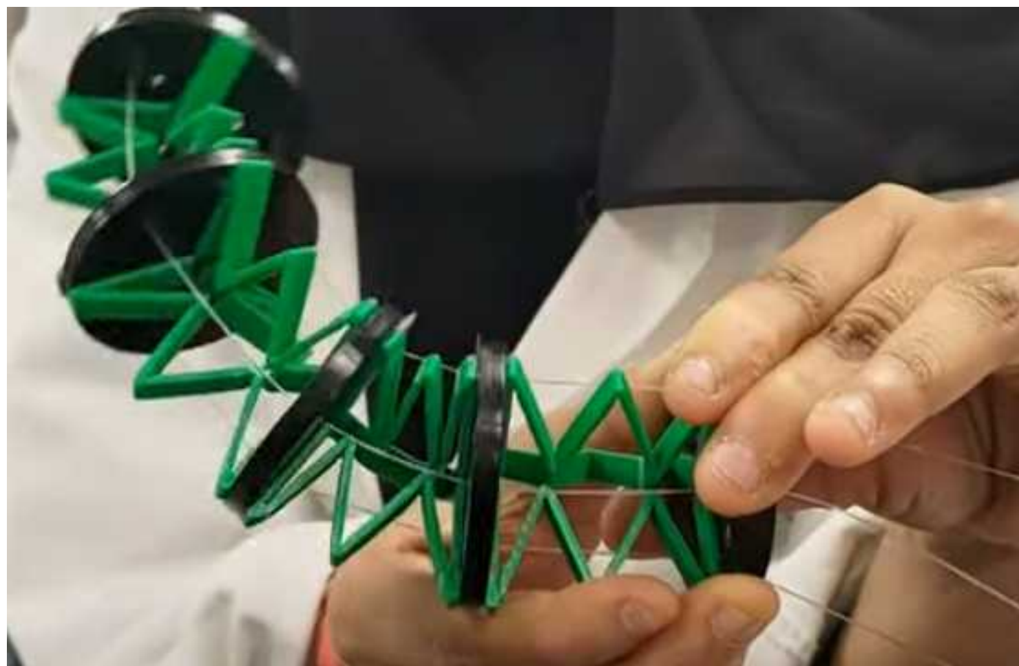
The first compliant springs had sharp bends that broke
