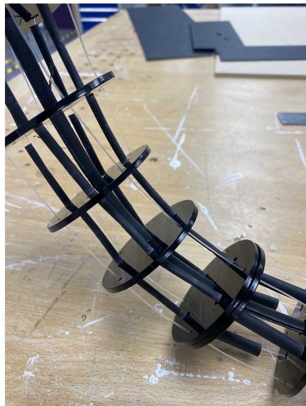
A tendon and sheath system was trialled but sheaths were too flimsy to be useful
