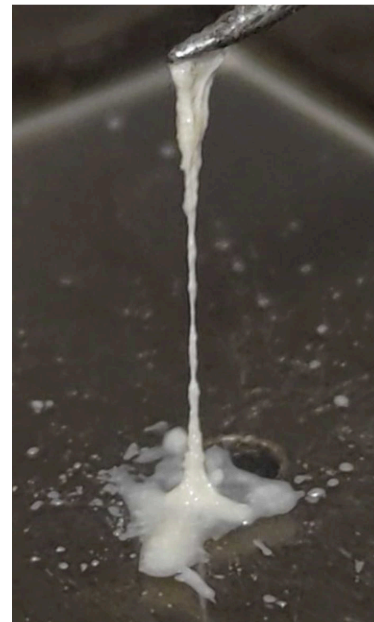
My attempt at creating fibres, hypothesising crosslinking of reactive end groups with heating.
