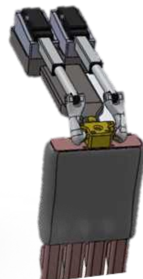
360° dual linear actuator wrist mechanism inspired by teslabot
